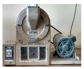
Fig. 3. Abrasive type polisher
