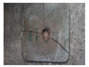
Fig. 4. Specimen showing failure of B40 after impact-endurance test
