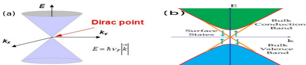
Fig. 1. (a) Dirac point showing touching of conduction and valence bands in graphene E - k diagram. (b) Topological insulator band structures with gapped bulk states and spin-filtered (up and down spins are indicated by \uparrow and \downarrow arrows) conducting edge/surface states
