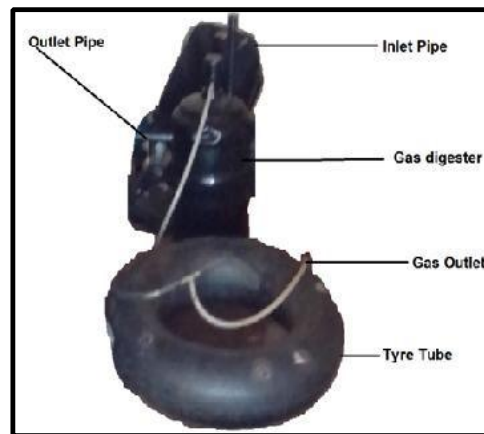
Fig. 1. Prototype of mini biogas digester In the experiment we tested the mini size biogas plant using slurry derived from cow dung with the addition of starter. The digester is placed at a room temperature of 30°C. Also, we use silica gel as starter for producing biogas.
