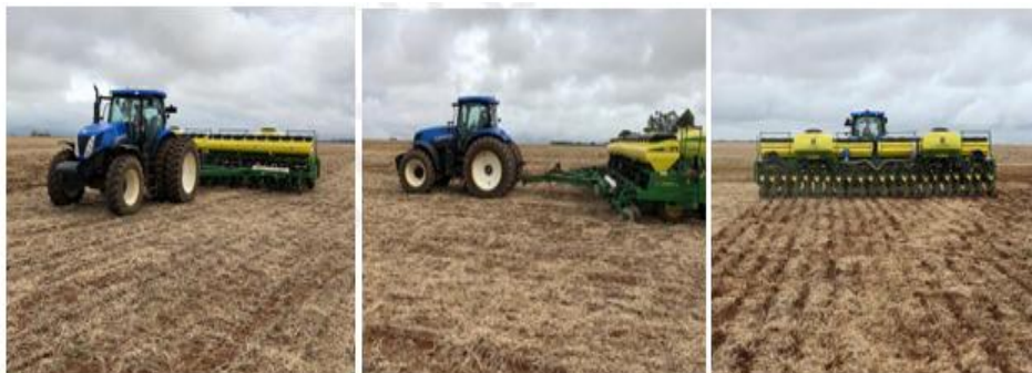
Fig. 1. Frontal, lateral and posterior views of the tractor-sowing system, used in sowing of corn
