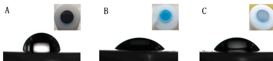
**Figure 1.** Images of contact angles of water drops deposited on GCE (A),  $\text{EGO}^{1/1.75\text{V}}$  (B), and  $\text{EGO}^{1/1.75\text{V}}_{2/-0.85\text{V}}$  (C).
