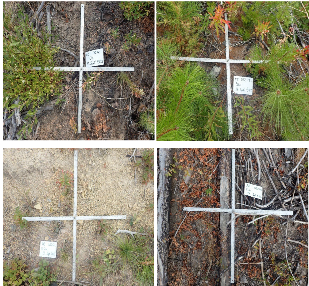
Figure 2. Ground cover photos from Copper King Unit 12 ( top row ), Sunrise Unit 22 ( bottom right ), and Rice Ridge Unit 26 ( bottom left ) in September 2022. These photos represent typical ground-cover conditions from the most disturbed unit we sampled on each fire; bare soil ranges from 6% to 60%. The time since salvage logging was more than four years for the Copper King unit, and three years for the Rice Ridge and Sunrise units.
