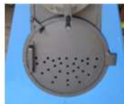
Fig. 2 Semi-perforated door of combustion chamber
