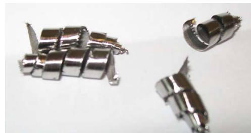
Fig. 8. Shape of chips obtained at turning titanium alloy by a helical tool
