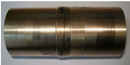
Fig. 9. Machined sample - turning by helical tool (left) and by tool of tip radius 0.4 mm
