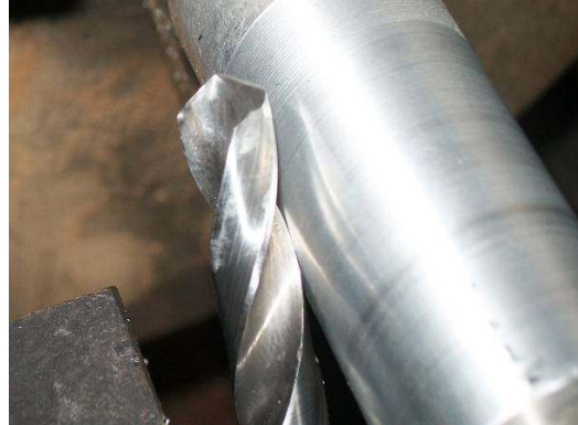
Fig. 3. Position of tool cutting edge regarding the workpiece
