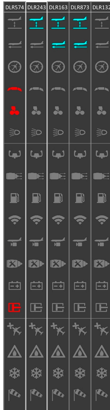
Figure 2. Icon display of the U-FLY GCS during a hydraulic pump failure for the RPAS-labeled DLR574, leading to the inability to deflect flaps and the landing gear, which is indicated by the red hue of the corresponding icons.
