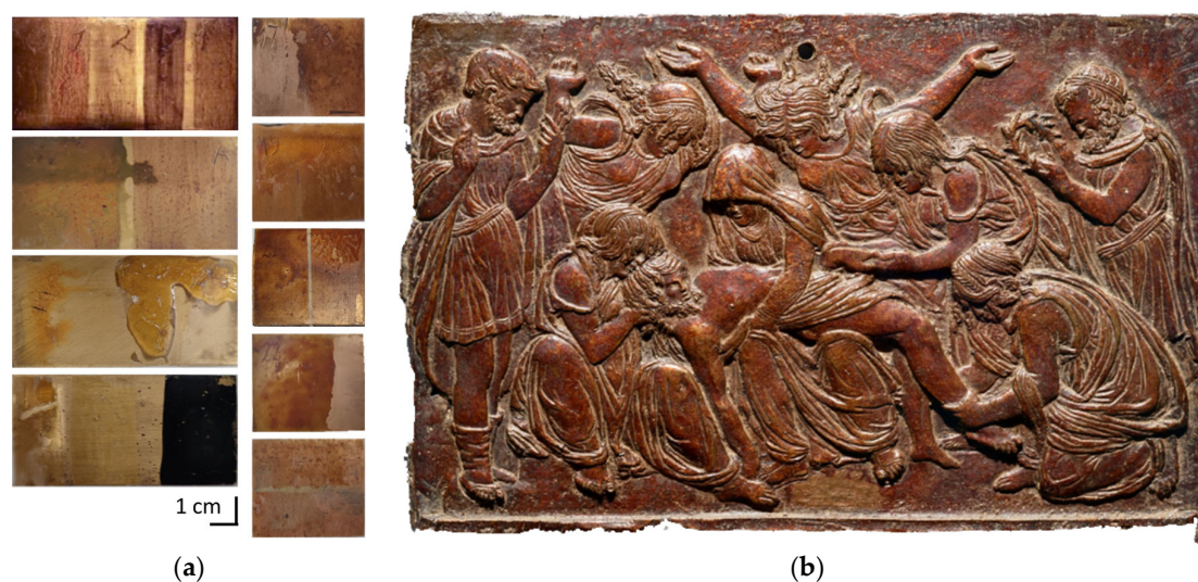
Figure 1. (a) Set of mock-ups made following historical recipes of organic coatings on copper-based alloy, and (b) Lamentation on Dead Christ, Bertoldo di Giovanni, bronze relief, 20 cm × 13.5 cm, Museo Nazionale del Bargello, Firenze.
