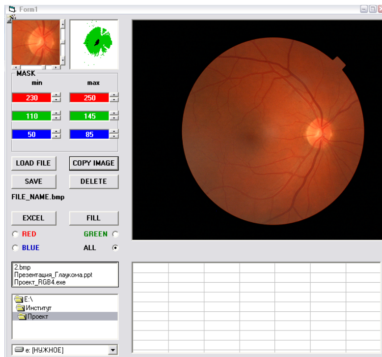
Fig. 1 The program interface. The top right window is the initial image; the small top left windows display the OD area and the result of its processing with the program. Below them the windows for the input of the colour mask values are seen. The rest elements are used for the interface between the program and the environment.
