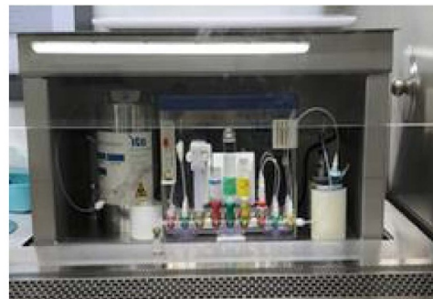
Centre 3: Synthesis performed in completely shielded LAFC (when the drawer is lowered below the surface of the cabinet).
